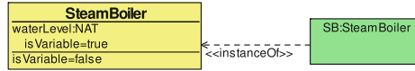
Fig. 5. steam_boiler_controller_domain_model: ontology associated with the root level of the goal diagram of Fig. 2
