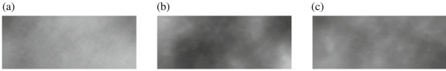
Fig. 11 Action visualizations for the poor policy. The forward action visualization shows that only the forward action is most probable. All actions have roughly equivalent action visualizations, indicated by the “murky” figures. (a) Left action. (b) Forward action. (c) Right action
