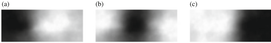
Fig. 10 Action visualizations for the good policy. The drone learns that when the camera is occluded (dark spots), it should move in the direction of the occlusion. (a) Left action. (b) Forward action. (c) Right action
