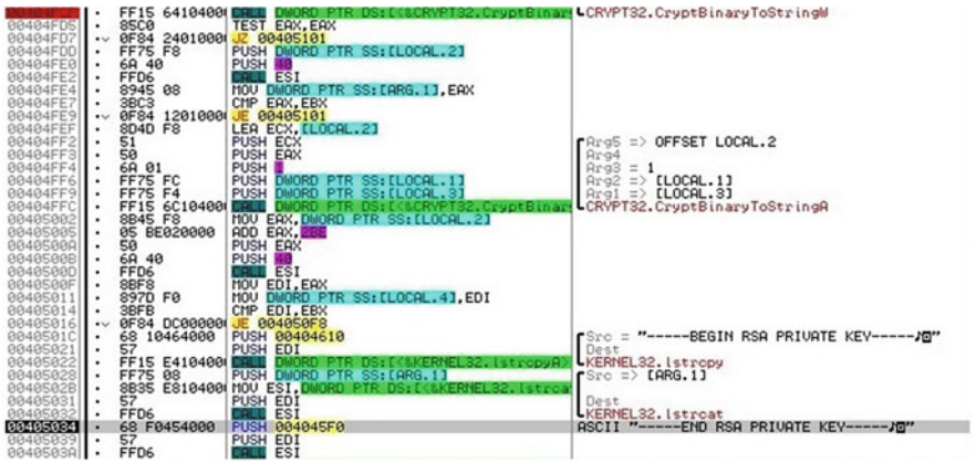
Fig. 9 RSA key is Base64 encoded
