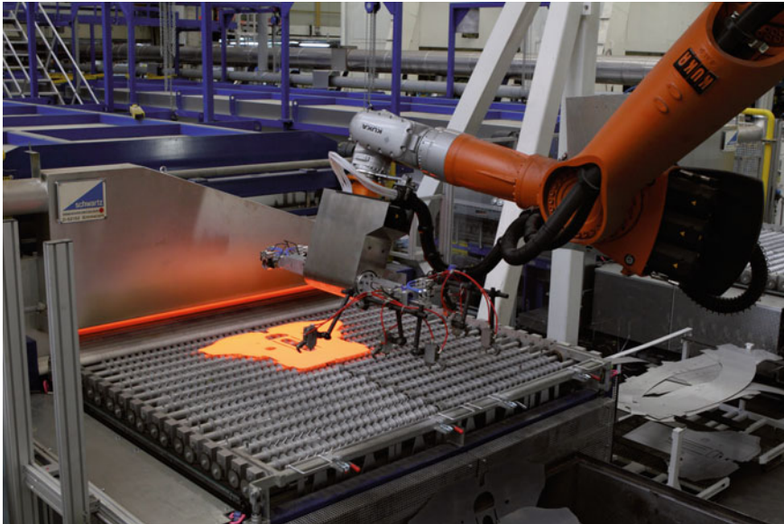
Fig. 5.5 Exit area with blank centering [7, 9]
