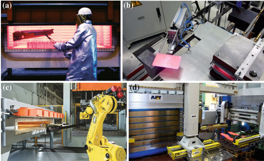
Fig. 5.13 Material handling systems: a manual handling [50], and b simple robot [18] are used for low volume production or tryouts; c industrial robot [51], and d linear feeders are used in mass production
