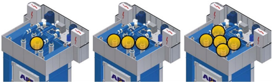
Fig. 5.19 Hydraulic “gearbox” activating the five cylinders in steps following the actual need of press force
