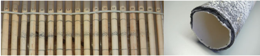
Fig. 5.4 AlSi coating builds up on ceramic rollers, if the blank is directly in contact with the rollers [7]
