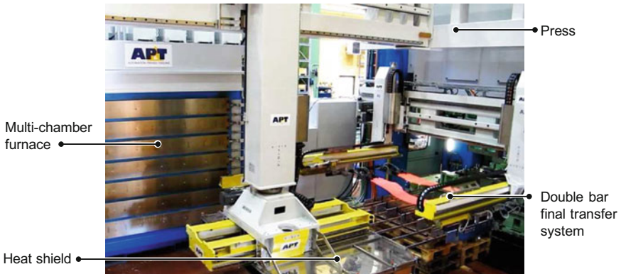
Fig. 5.15 Material handling inside a heat shield as far as possible followed by handling with transfer feeder with two blanks at a time. The double-bar transfer system minimizes the time in open air
