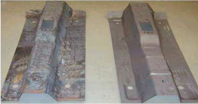
Fig. 3.7 VW Passat transmission tunnel stamped using: a uncoated blank causes scales; b coated blank has no scale problems [18]
