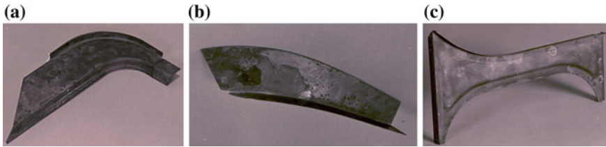
Fig. 3.3 Various geometries to study formability: a Stretch flanging, b Curved flange, c Stretching [4]
