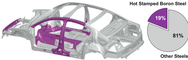
Fig. 3.10 Hot stamped boron steel components in Passat B6 (SOP 2005) [30]
