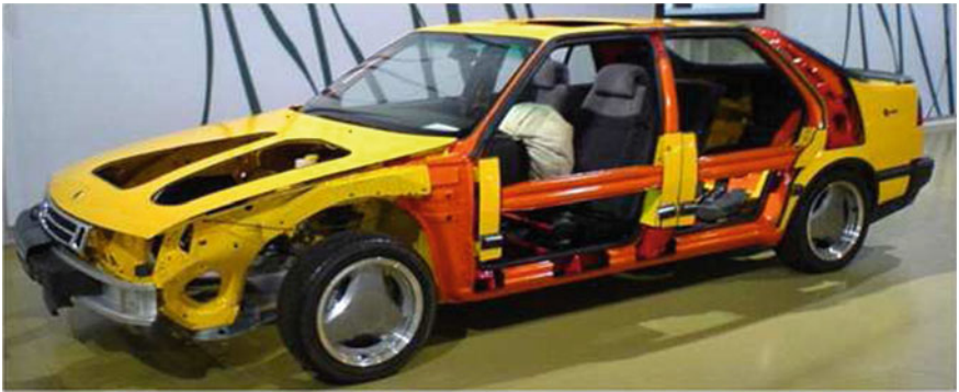
Fig. 3.6 1984 Saab 9000 was the first automobile to have hot stamped side impact door beams [image from http://wikipedia.org ]
