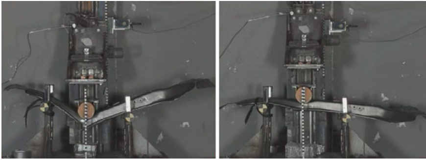
Fig. 8.40 Three-point drop test results at same energy level: a fully hardened B-pillar, spot welded along the flanges, b B-pillar with tempered and spot welded flanges [2]
