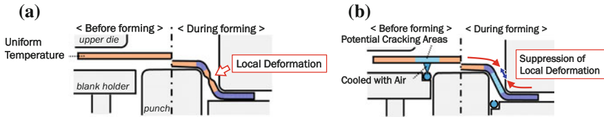
Fig. 6.27 Comparison of the partial cooling technique with conventional hot stamping technique [60]
