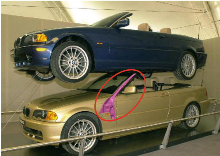
Fig. 3.9 One of the earliest examples of A-pillar reinforcement in BMW 3 Convertible (E46, SOP 2000) (Image re-created from [19])
