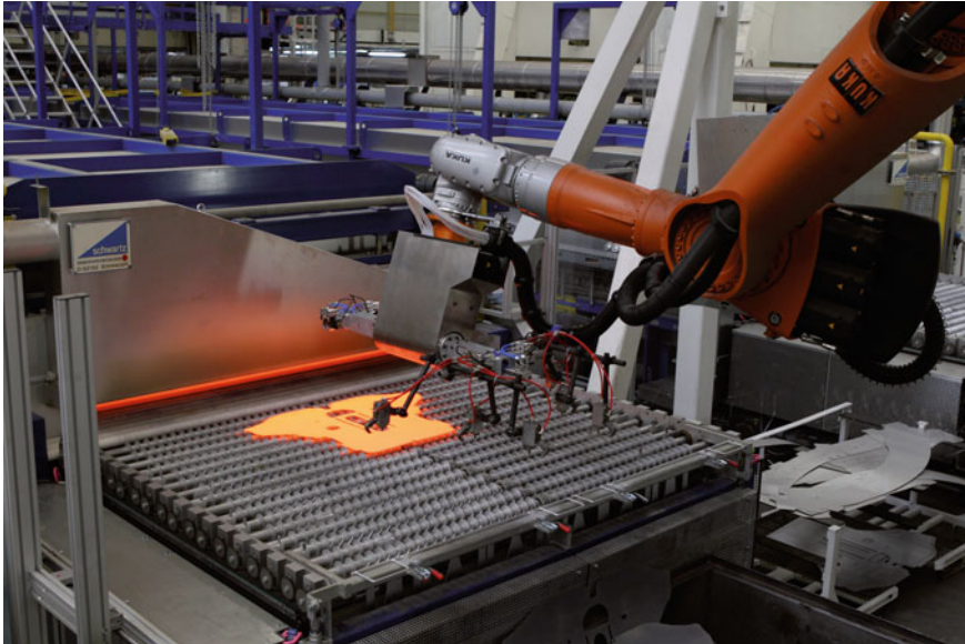
Fig. 5.5 Exit area with blank centering [7, 9]
