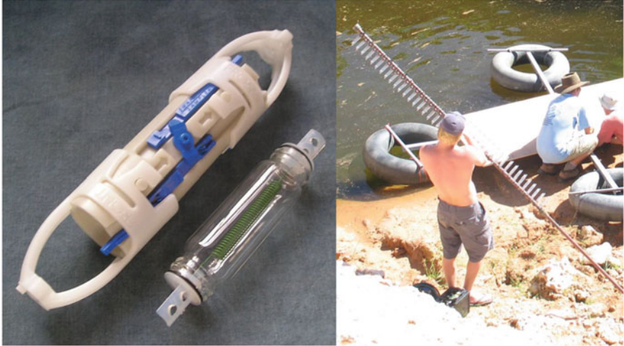
Fig. 24.1 Snap Samplers ® can be chained to take simultaneous samples of undisturbed water from different depths. Image courtesy of Sandy Britt, ProHydro, Inc. (left); pneumatic sampler taking simultaneous samples at 5 cm intervals over a depth of 3 m (Seymour et al. 2007). Photo by © William F Humphreys (right)
