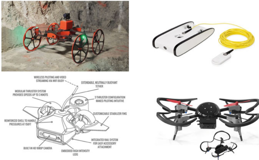
Fig. 24.2 Clockwise from top left. 1 TILT Ranger ( http://inkonova.se/tilt-ranger/ ) is rugged, flies, climbs and swims and can carry a payload ( https://www.youtube.com/watch?v=XSTfsJWz7RY ); 2 Trident underwater remotely operated vehicle (ROV) is compact, 410 mm long, and dives to a depth of 100 m with a 3–4 h duration ( https://www.youtube.com/watch?v=rnVpXb_1RhA ; https://www.openrov.com/products/trident/#specs ); 3 Small underwater ROVs are being fitted with equipment racks that will increase their task diversity ( https://www.fathomdrone.com/ ); 4 Aerial drones, such as Micro Drone 3.0, can be tiny, avoid collisions and fly into fine spaces to take stabilised HD video ( https://microdrone.co.uk/products/micro-drone-3plus , https://www.google.com.au/search?q=Micro+Drone+3.0.+Stabilised+HD+video.&rlz=IC1CAF_enAU610AU610&oq=Micro+Drone+3.0.+Stabilised+HD+video.&aqs=chrome..69i57.647j0j8&sourceid=chrome&ie=UTF-8 )
