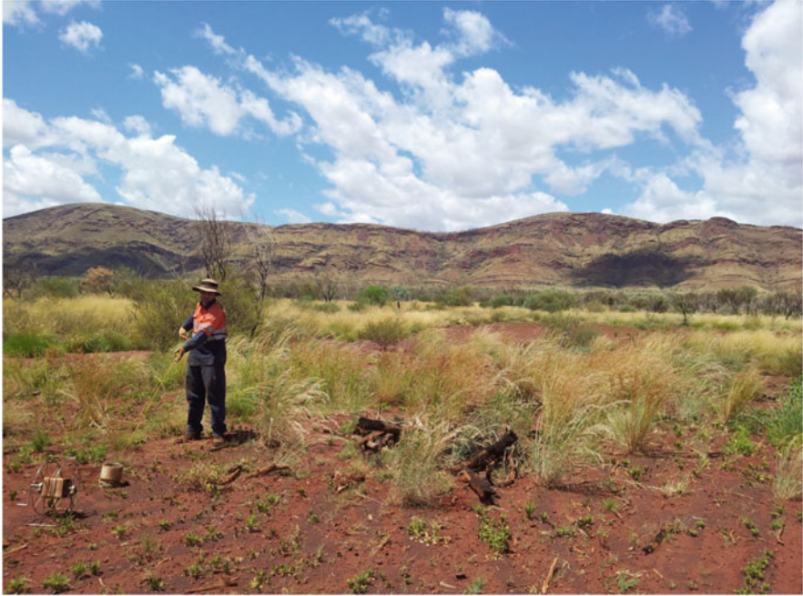
Fig. 23.1 Drill hole being sampled for troglofauna by scraping. Hole has short PVC collar to prevent collapse at the surface and a metal “sleeve” has been inserted in the collar to reduce friction when retrieving the sample. Deeper sections of the hole are uncased
