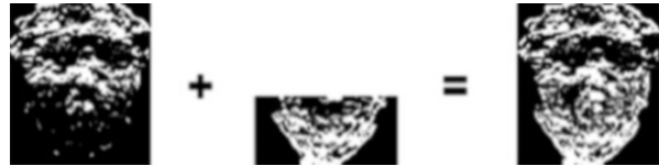
Fig. 5.23 Sum of downward and upward gradients to locate the eyes
