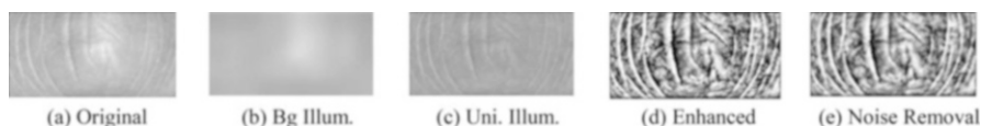
Fig. 16.22 Local CLAHE-based FKP enhancement. (a) Original. (b) Bg illum. (c) Uni. illum. (d) Enhanced. (e) Noise removal
