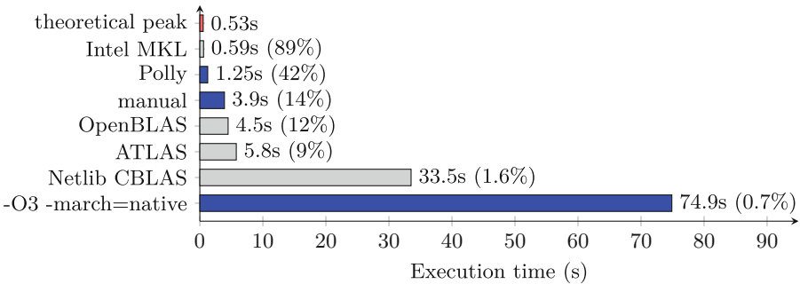
Fig. 2. Comparison of matrix-multiplication execution times on an Intel Core i7 7700HQ (Kaby Lake architecture), 2.8 GHz, Turbo Boost off
