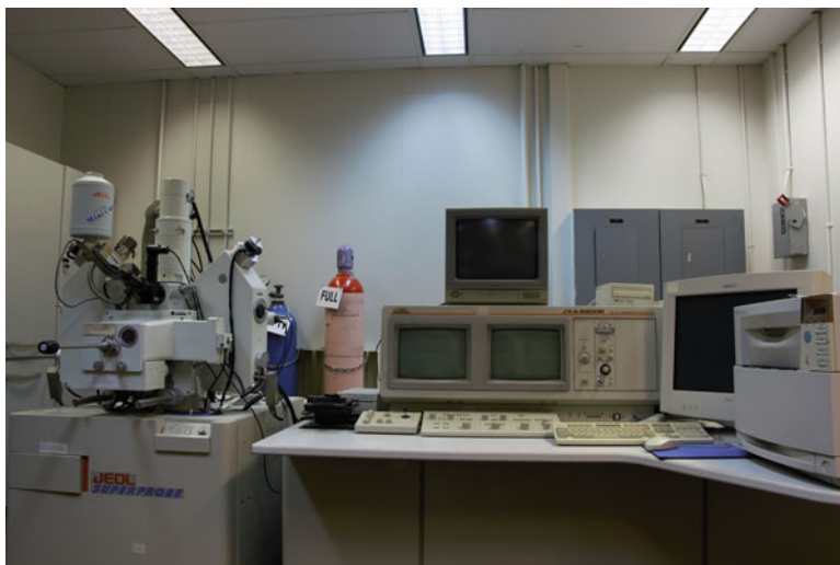
Fig. 7.18 Photograph of electron probe microanalyzer (EPMA) fitted with two wavelength dispersive (WD) x-ray spectrometers
