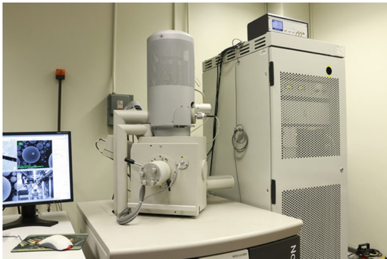
Fig. 2.1 Photograph of a typical SEM with electron column, specimen chamber, and electronics/ computer control system
