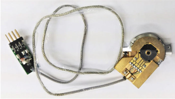
Fig. 2.34 Photograph of backscattered electron (BSE) detector along with associated electronics. The BSE detector is the dark wafer chip with a hole inside to allow passage of electrons. The chip is fixed on the brass mount. Four quadrants are visible on the chip
