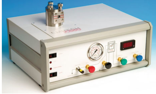
Fig. 8.24 Photograph of critical point dryer. (Courtesy of Quorum Technologies)
