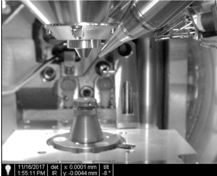
Fig. 2.29 Photograph of the inside of the specimen chamber showing objective pole piece at the top and specimen stage and holder at the bottom. Immediately to the right-hand side of the pole piece is the collimator attached to the front of EDS detector. The upper rightmost section shows E-T detector with the front end covered by Faraday cage to attract low-energy secondary electrons emanating from the specimen surface
