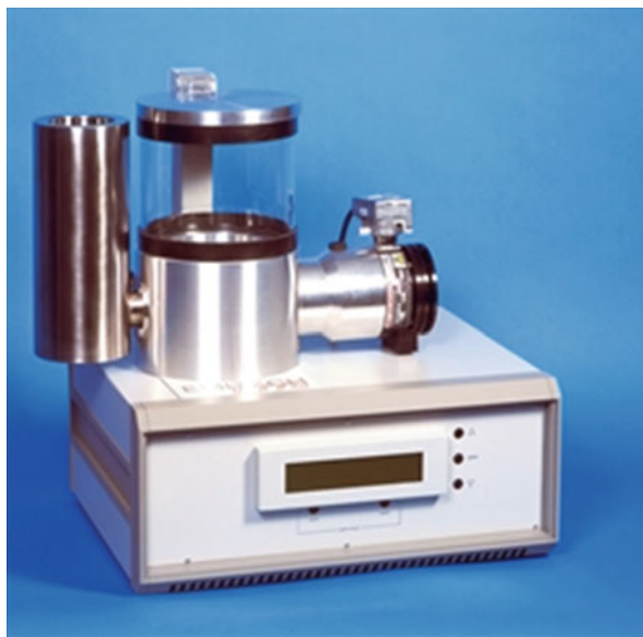
Fig. 8.23 Photograph of a liquid nitrogen cooled freeze dryer. (Courtesy of Quorum Technologies)
