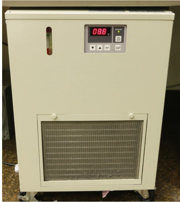
Fig. 2.41 Typical water chiller used to remove heat from various components of the SEM
