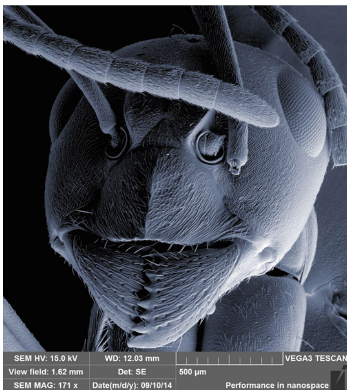
Fig. 1.5 Secondary electron SEM image of an ant showing detailed three-dimensional details. (Image courtesy of TESCAN)
