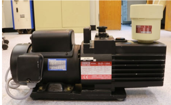
Fig. 2.39 Photograph of a typical rotary pump
