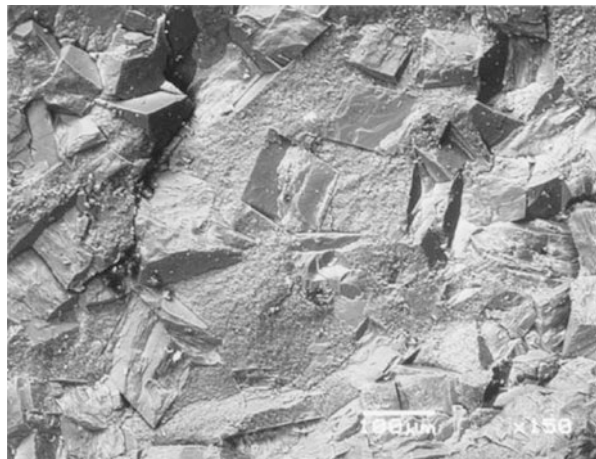
Fig. 8.15 Secondary electron SEM image of a coated carbonate rock sample
