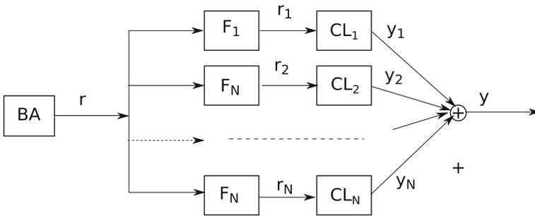
**Fig. 7** Part of an open-loop coordination architecture for an aggregate of LCVDs to track a grid-level VES reference. Only the forward path between the BA and the loads are shown; the outer loop feedback between the “Grid” block of Fig. 4 and the BA is omitted
