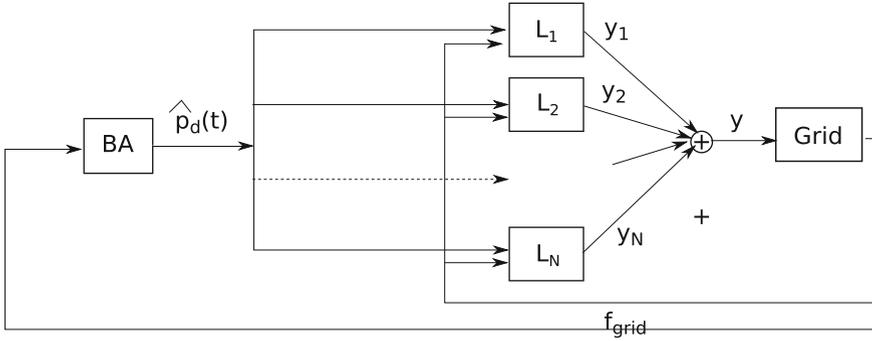
**Fig. 8** A potential control architecture for coordination among VES resources by using local feedback (on grid frequency  $f_{grid}$ ) and broadcast from BA on the predicted demand–supply imbalance  $\hat{p}_d$
