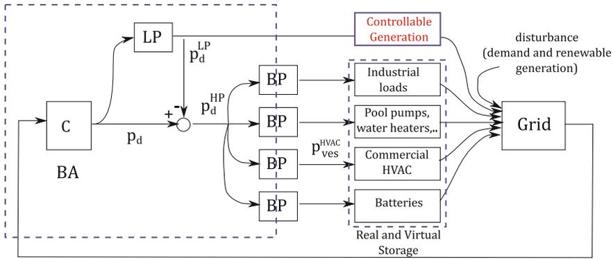
**Fig. 4** A potential control architecture for the smart grid with VES based on spectral decomposition. The “Grid” block represents everything other than controllable generation and storage resources, such as loads (baseline), transmission and distribution networks, etc.
