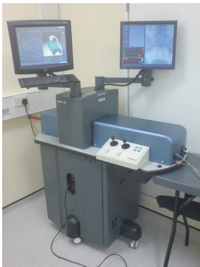
Fig. 7 The ANGIO Mentor™ Ultimate endovascular trainer has a similar range of arterial procedures as the VIST™ with more advanced haptic technology. The ANGIO Mentor™ Express and ANGIO Mentor™ Mini have similar simulation packages but with less peripheral attachments such that the Mini can be transported in a handheld case
