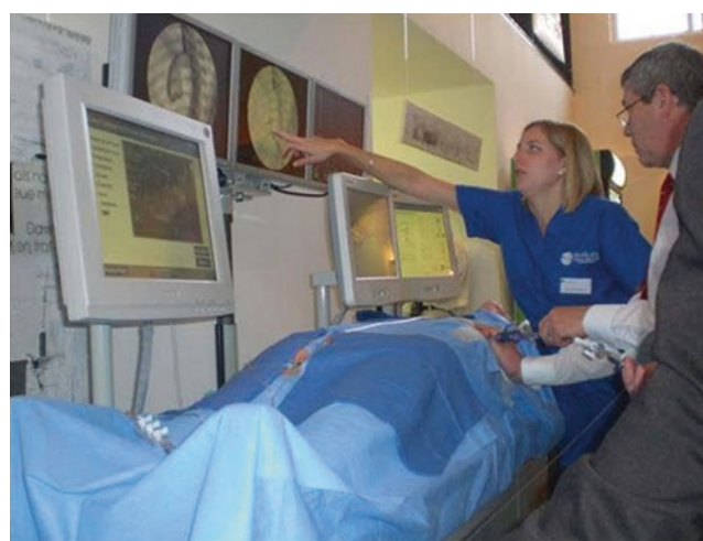
Fig. 8 The SimSuite simulator provides tactile “haptic” feedback and displays real-time imaging and physiologic information
