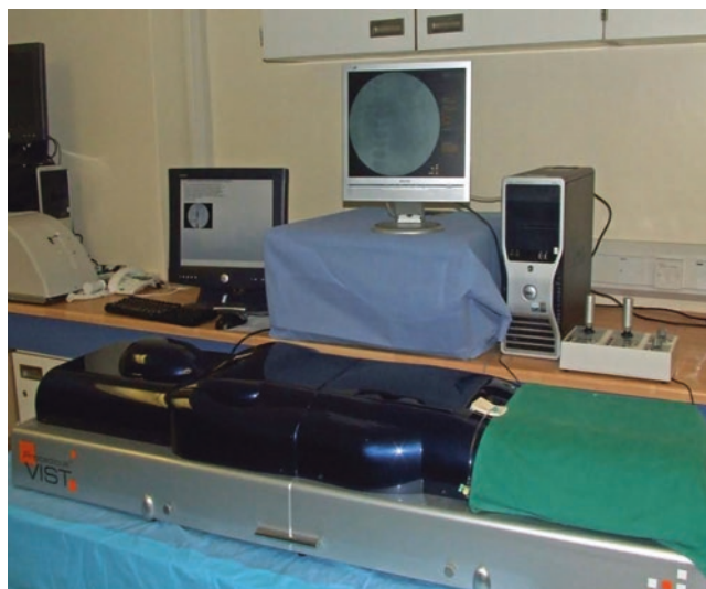
Fig. 6 The Procedicus Vascular Intervention System Training (VIST™) simulator comprises a mechanical unit housed within a plastic mannequin cover, a high-performance desktop computer, and two display screens. Modified instruments are inserted through the access port using a haptic interface device. Performance is measured using metrics such as volume of contrast used, fluoroscopy time, and markers of stent placement accuracy
