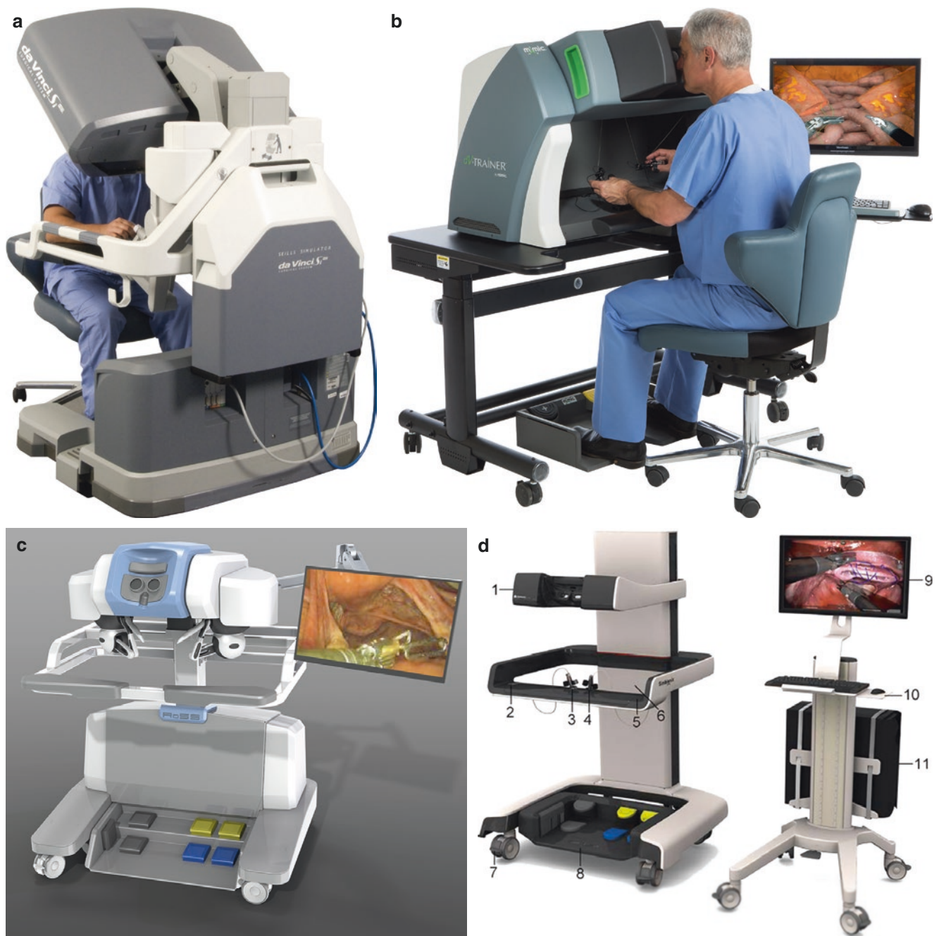
Fig. 2 Robotic VR simulators: da Vinci Skills Simulator, dV-Trainer, RoSS, and RobotiX Mentor. (With permission of Intuitive Surgical Inc., Mimic Technologies, Simulated Surgical Systems, and 3D Systems, formerly Simbionix [5, 7–9])
