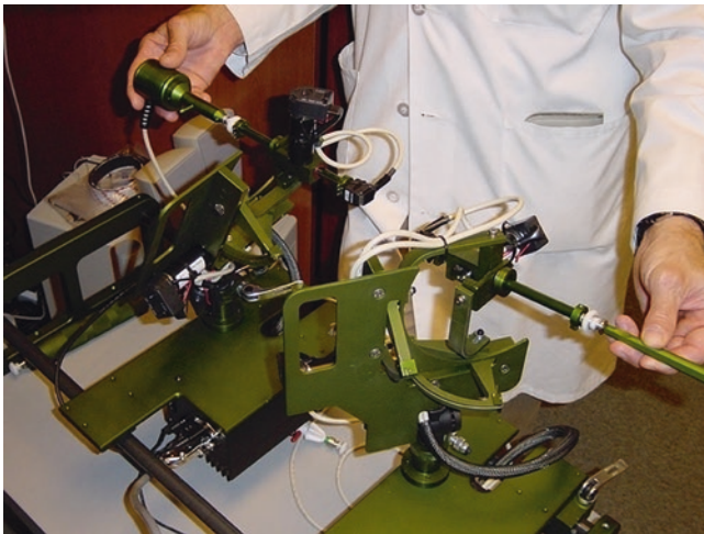
Fig. 5 Shoulder arthroscopy simulator ca. 1997 Prosolvia
