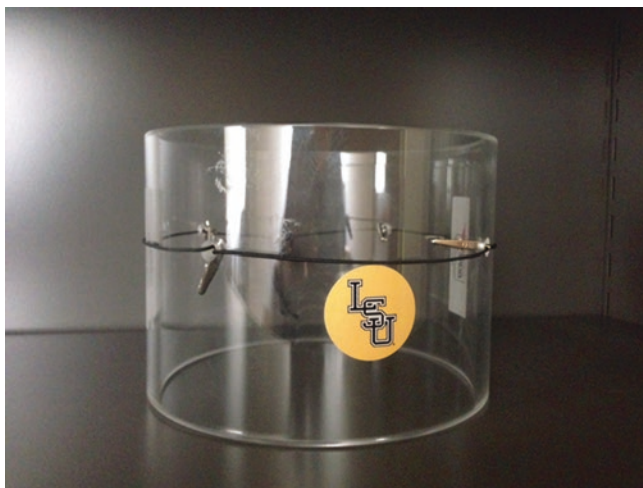
Fig. 11 Plastic tube in which the clockface model is secured to simulate the depth of the abdominal cavity
