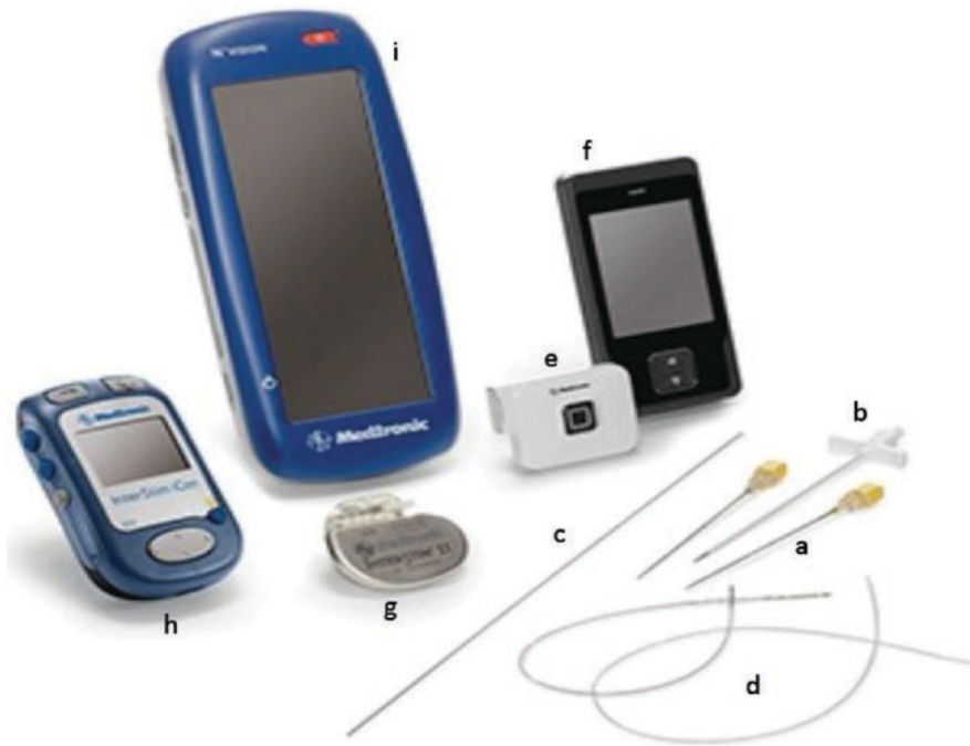
Fig. 8.8 The equipments required for SNM: (a) needles; (b) introducer sheath; (c) directional guide; (d) tined lead electrodes; (e) external test stimulator, verify; (f) controller for verify; (g) InterStim II 3058; (h) InterStim patient programmer iCon; and (i) N'Vision programmer
