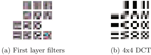
Fig. 3. Some of the first layer filters display visual similarity to a spatial representation of the 4x4 DCT transform used in H.264/AVC
