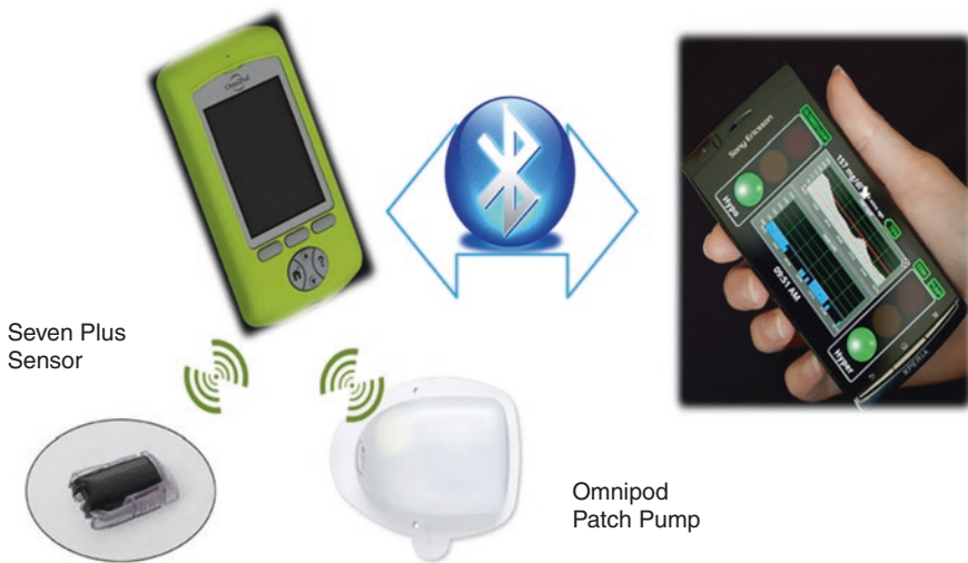
Fig. 6.1 First prototype of wearable artificial pancreas system used in home-like setting by patients with type 1 diabetes. Subcutaneous insulin infusion is delivered by an OmniPod (Insulet, Boston, USA) wirelessly connected to a handheld relay (‘green box’) which receives glucose sensor signal (Seven Plus, Dexcom, San Diego) from CGM transmitter (lower left hand side device) and transmits by Bluetooth the glucose signal to the smartphone-based Diabetes Assistant (DiAs, University of Virginia), on the right hand side. The closed-loop algorithm is run by the DiAs, which includes a patient interface displaying information of sensor glucose values, insulin delivery rate and two traffic light icons presenting detected risks of hypo- and hyperglycaemia, respectively. The control algorithm modulates insulin infusion by Bluetooth-mediated signals to the relay box
