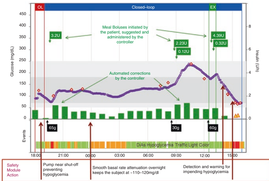
Fig. 6.2 Display of closed-loop control of blood glucose by subcutaneous insulin infusion through a model predictive control algorithm run by the Diabetes Assistant (DiAs) smartphone-based platform. This information is provided by the remote control server from 3G key transmission from the DiAs smartphone. The arrows indicate the meaning of displayed data
