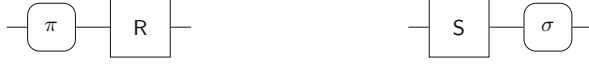
Fig. 1. The real (left) and the ideal (right) setting considered in indifferentiability. We depict resources using rectangular boxes and converters using rounded boxes. The honest party’s interface is depicted on the left, and the dishonest’s on the right side.
