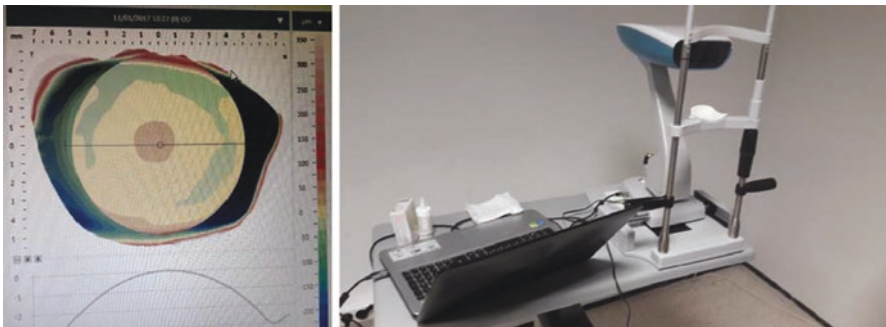
Fig. 28.9 System for the characterization of corneo-scleral geometry ESP (Eye Surface Profiler, Eaglet-Eye). Right, general aspect of the device; left, aspect of the main screen showing the map obtain in a specific case measured with the device
