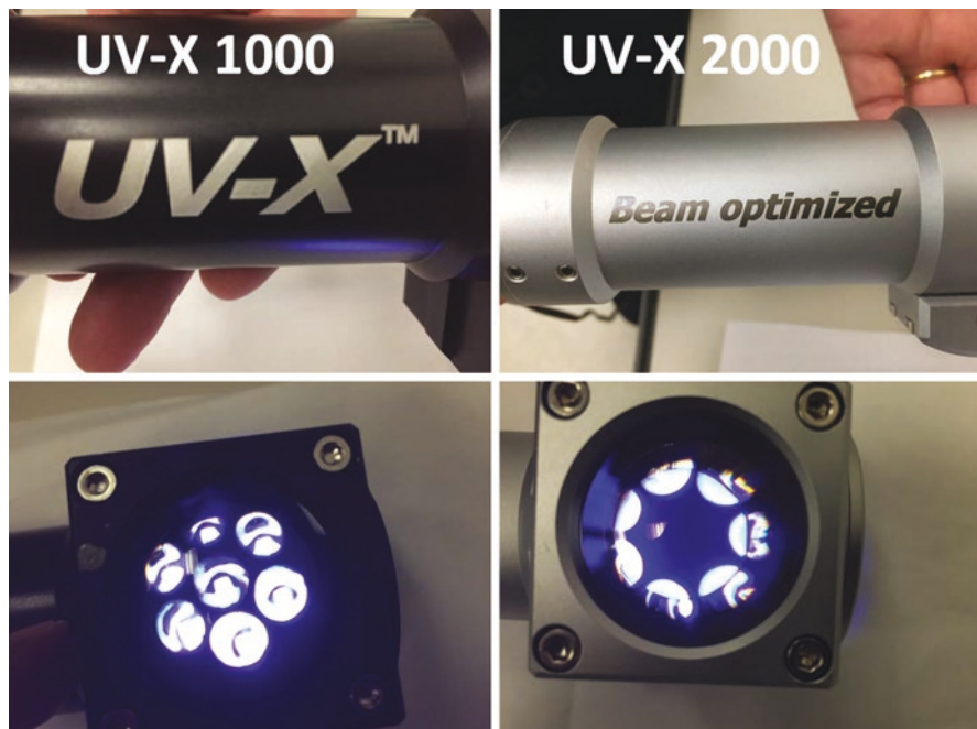
Fig. 16.7 The UV-light sources both comprise 7 Light-emitting diodes (LEDs) but the LEDs are arranged differently. On the left, the UV-X 1000 has 7 LEDs that fill the aperture with 1 LED in the centre and 6 LEDs in the periphery and on the right, the 7 LEDs are arranged with a gap in the centre and 7 LEDs in the periphery
