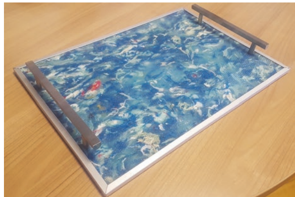
Fig. 2.3 Textile waste–reinforced composite tea tray created by Yalcin et al. (2012). This tray, composed of 100% cotton knitted and woven fabric production waste and a polypropylene matrix, is produced by a compression molding technique. (Reproduced from Yalcin et al. (2012), with permission)
