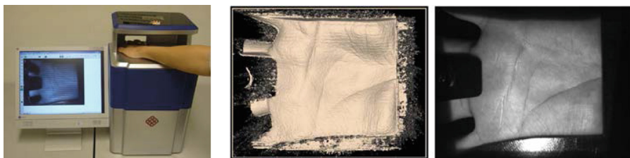
Fig. 1. The existing 3D palmprint measurement systems.
