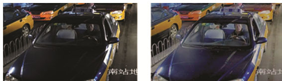
Fig. 7. MSRBVC algorithm test results: (left) original frame, (right) enhanced frame.
