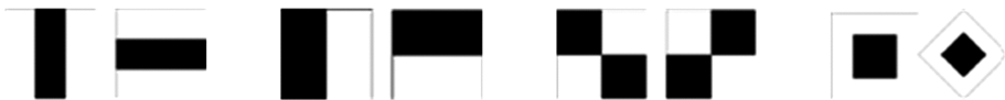
Fig. 1. Common Haar features: (picture 1) Linear feature, (picture 2) Edge feature, (picture 3) Diagonal feature, (picture 4) Central feature.
