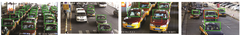
Fig. 4. Preliminary detection results of window area.
