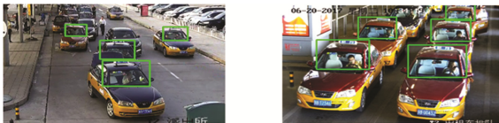
Fig. 6. Secondary detection results of window area.
