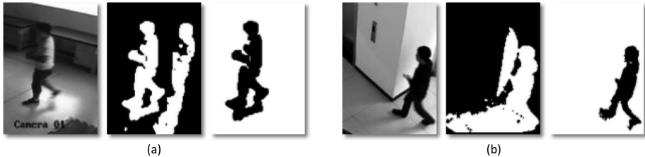
Fig. 2. Motion area extraction sample of modified ViBe method. (a) ghost remove, (b) shadow remove.
