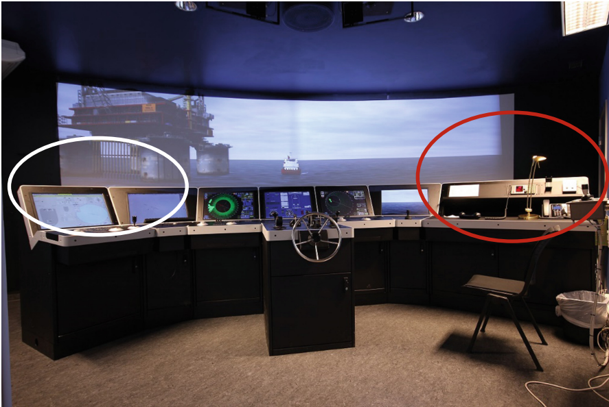
Fig. 1. Dynamic positioning operational systems (white circle) and communication systems (red circle) in Ocean Training & Competence AS (OTC) simulator (Color figure online)
