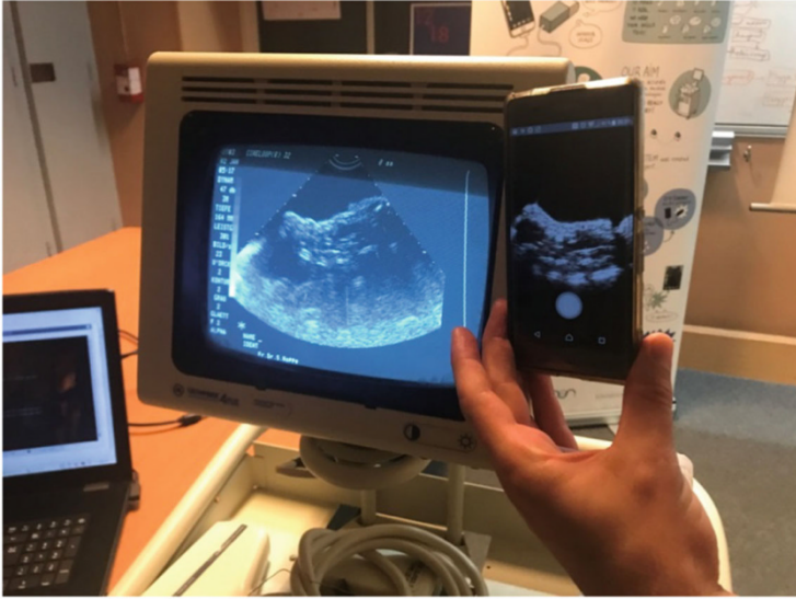
Fig. 1 Comparison of a console style ultrasound device (left) with the recently developed portable open source ultrasound imaging device EchOpen that can be operated together with a smartphone (right). (illustration by courtesy of EchOpen )
