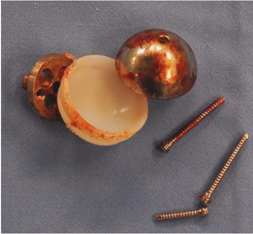
Fig. 19.15 Photograph of a retrieved RSA (implantation time: 7 years); retentive polyethylene humeral insert rim damage due to bony scapular impingement or screw contact
