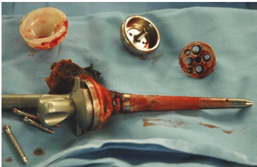
Fig. 19.20 Retrieved RSA implanted in a 73-year-old female with rotator cuff insufficiency, revised after 4 years for humeral stem loosening. Damage of the modular humeral junction consisted of mild to moderate fretting of the stem
