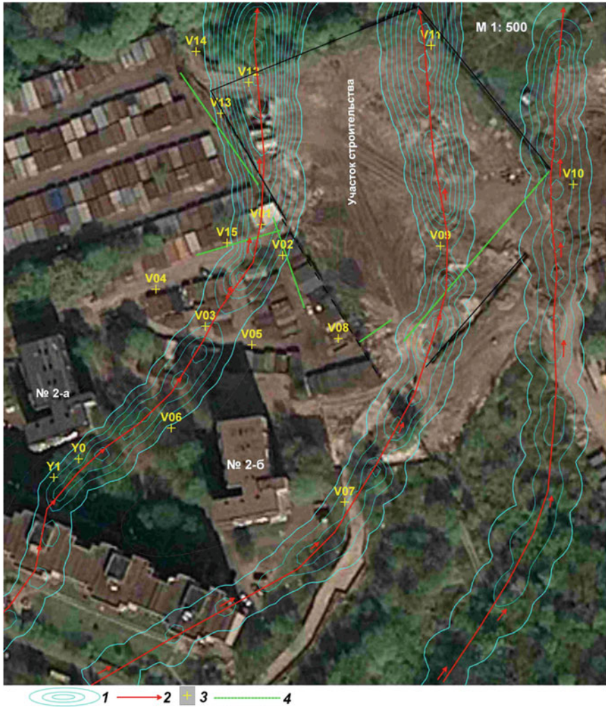
Fig. 31.5 Map of soil moistening areas and migration routes of underground water flows at the site of a residential complex construction on the satellite image of area. 1—zone of soil moistening; 2—direction of groundwater migration; 3—VERS points; 4—profiles of GPR sounding
