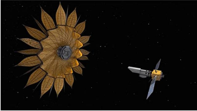
**Fig. 12.1** The starshade has to be tens of meters across and fly in exact formation with a space telescope that is several tens of thousands of kilometers away. Compared to previously used technologies, much more information could be obtained regarding the planet's atmosphere and whether an observed exoplanet is potentially habitable. *Credit: NASA*
