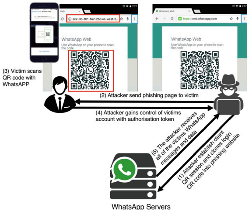
Fig. 10 WhatsApp QR link hijacking attack (initiated via sending a target victim a phishing website link). Here the spoofed QR code is automatically refreshed through the Javascript that has been copied from the legitimate WhatsApp authentication page
