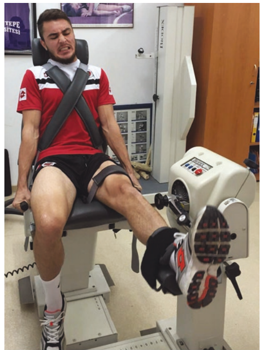
Fig. 44.2 Isokinetic strength tests should be performed to compare injured/non-injured side knee extensor/flexor torque ratios
