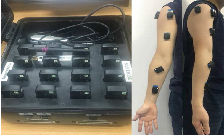
Fig. 1. Data collection device and electrode configuration.
