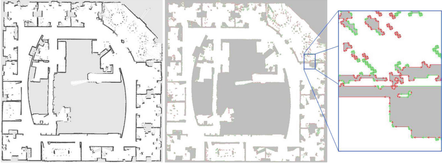
Fig. 7. Occupancy grid (left), full converted PolyMap (middle) and zoom in the PolyMap (right) (Color figure online)
