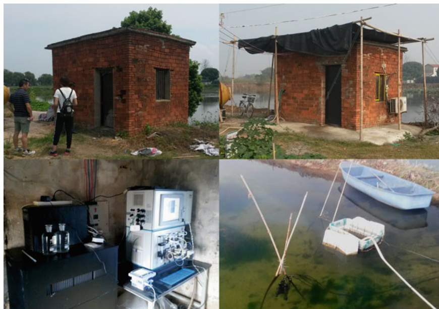
Fig. 5.25 Impressions from the field station at the Bao'an lake near Wuhan. Upper left and right: housing of the monitoring station before (June 2017) and after (November 2017) constructional upgrades. Lower left: view into the compiled monitoring station with Daphnia -Toximeter, IQ SensorNet controller, uninterruptible power supply and a backup data collector. Lower right: swimming basket with pump for raw water withdrawal and IQ SensorNet probes in an experimental pond of the field station (Source: M. Rybicki)
