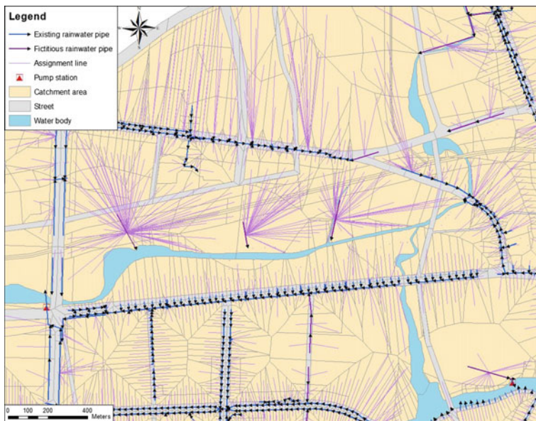
Fig. 3.26 Example of fictitious sewer network
