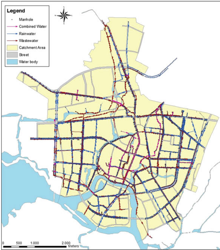
Fig. 3.17 Overview of sewer system in Chaohu city
