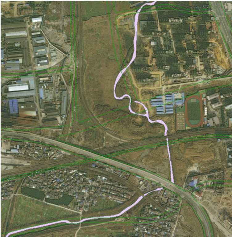
Fig. 3.4 Shuangqiao River bed structure (pink) in comparison to the old satellite images provided by ArcMap Basemap layer based on DigitalGlobe imagery from 2014
