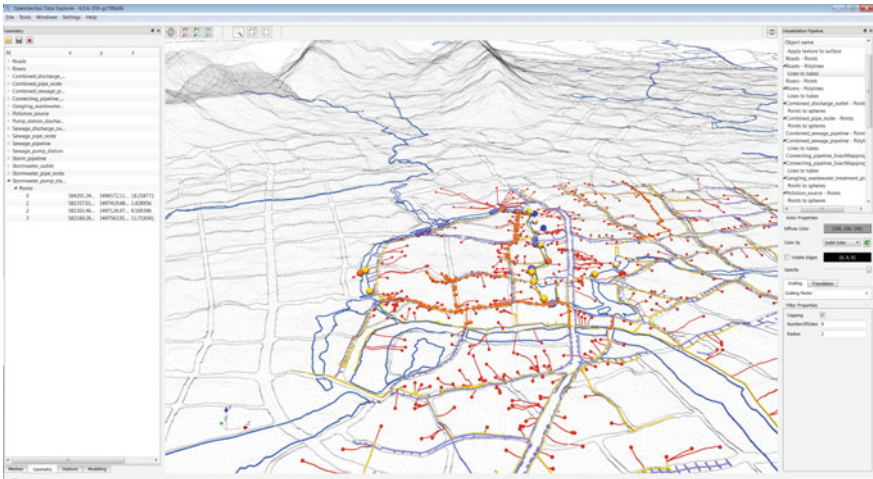
Fig. 6.16 Pre-processing of data sets. Depicted is the OpenGeoSys Data Explorer interface while integrating the drainage pipeline system in Chaochu City into the existing scene. The terrain surface mesh is semi-transparent visible in the background for reference as well as the road- (grey) and river network (blue). Fifteen data sets related to the drainage system have been loaded, mapped and assigned colours according to their function (e.g. violet data represents storm pipeline infrastructure, yellow signifies sewage infrastructure, etc.)
