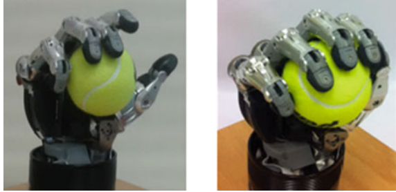
Fig. 4 Example of grasp configurations without ( left ) and with ( right ) the additional term based on the virtual object centroid
