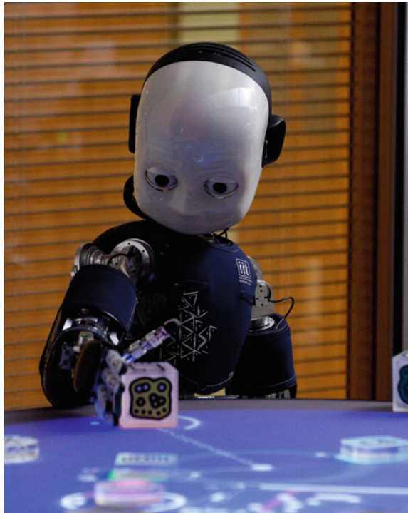
Fig. 1 The iCub humanoid robot. A biomimetic robot platform for embodied testing of theories of general human intelligence developed by European researchers led by the Italian Institute of Technology. Picture from Sheffield Robotics
