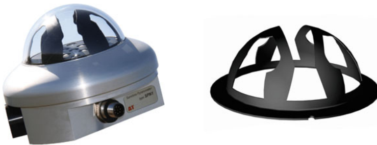
Fig. 24 A new concept for the measurement of global and diffuse irradiance with a shadow mask and without any moveable parts: SPN1 pyranometer by Delta-T. There is always at least one shaded and one unshaded sensor
