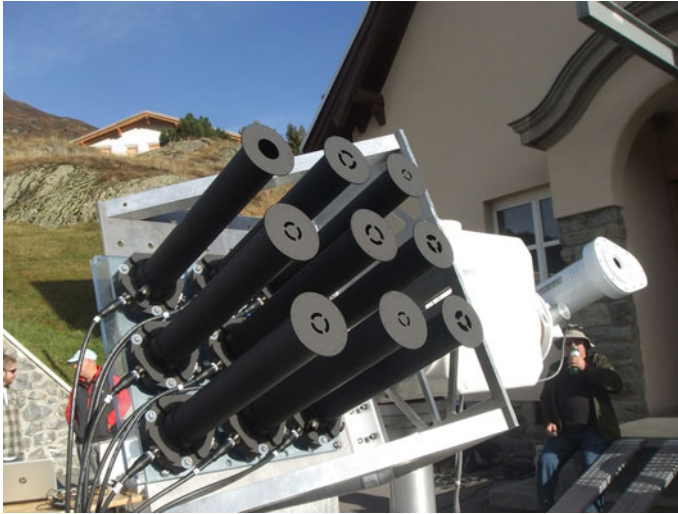
Fig. 16 Measurement of circumsolar radiation from the difference between DNI signal of partially shaded and unshaded sensors during IPC-XII in Davos, performed by Black Photon Instruments
