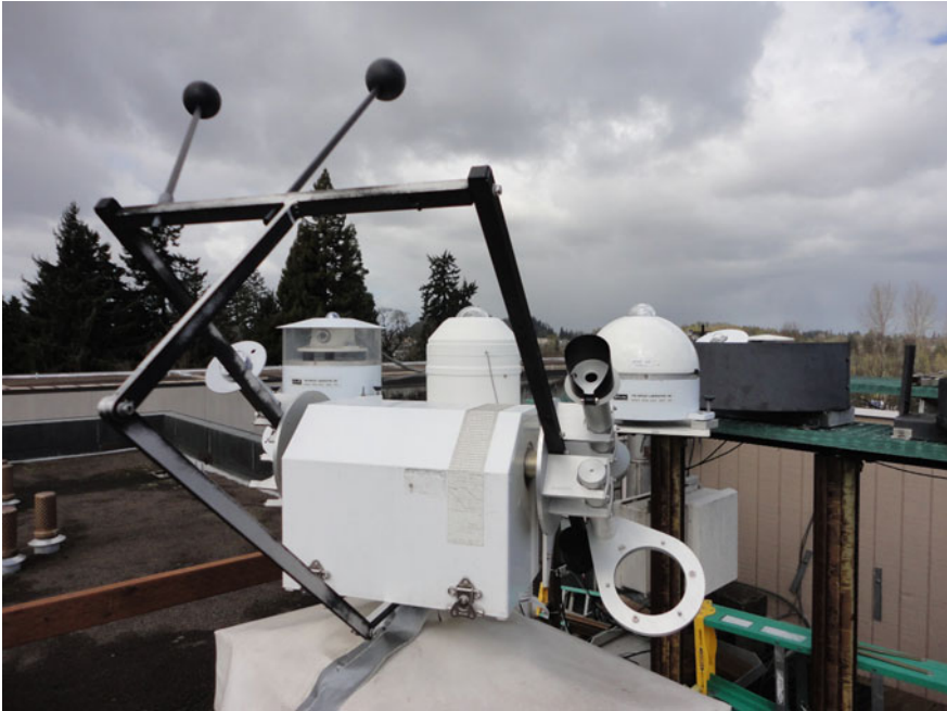
Fig. 8 Pyranometers, pyrgeometer, and pyrhemometers mounted on an automatic tracker at the UO SRML station in Eugene, Oregon. The pyranometers are in ventilators. The tilted pyranometer on the back shelf had a shade ring to provide a small but uniform ground-reflected component. Data loggers, AC power, and Internet connection are in the shack in the lower background. The very back shelf has room for other instruments to be calibrated. All pyranometer sensors are at the same level. The wind tower with anemometer and pyranometer to measure ground reflection, not shown in this photograph, are to the northwest out of the path of the sun. Photograph taken by Rich Kessler for the UO's Solar Radiation Monitoring Laboratory
