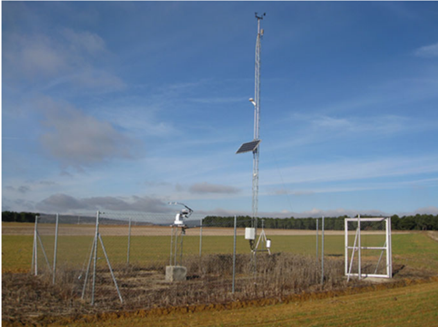
Fig. 2 Example of a meteorological and radiometric station protected with fencing to avoid intrusions. Geonica©
