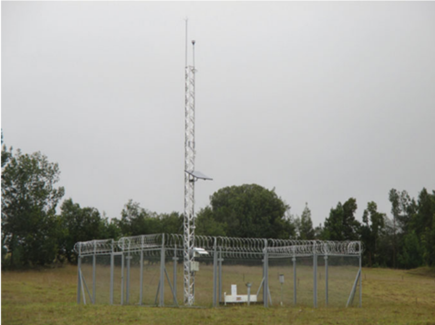
Fig. 3 Example of a meteorological and radiometric station protected with barbed fencing to avoid intrusions. Geonica©
