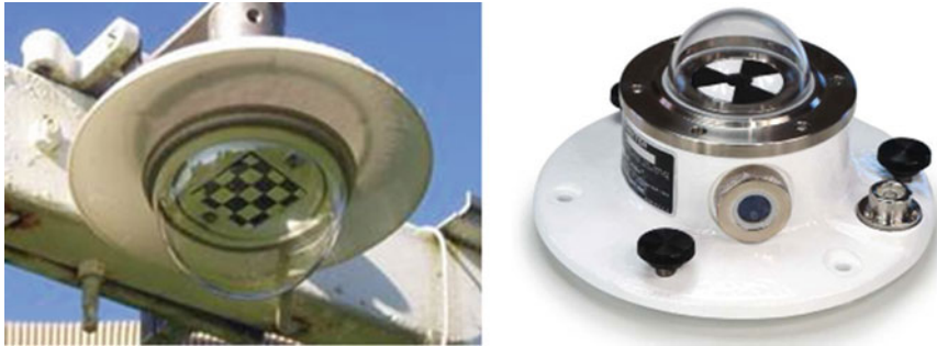
Fig. 2 Some examples of black-and-white pyranometers: (left) a Yanishevsky pyranometer used for albedo measurement, (right) an Eppley model 8-48 diffuse pyranometer
