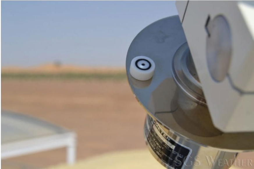
Fig. 4 Sunspot on target is slightly low and to the left. This is well within the tolerance of the pyrheliometer, but if the sunspot moves across the black ring of the target, the instrument needs to be realigned. Specification of the tracker indicates when realignment is needed
