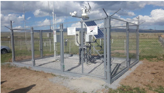
Fig. 16 Radiometric station developed in Armenia for the project utility-scale solar power project from the world bank. Courtesy of Geonica ©
