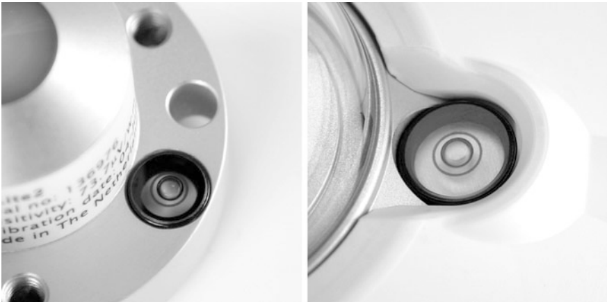
Fig. 5 The instrument on the level shows the bubble in the level to one side. The instrument should be releveled. The instrument on the right has the bubble inside the circle of the level. It is hard to get the bubble more centered than this example. One should test the sensitivity of the bubble level
