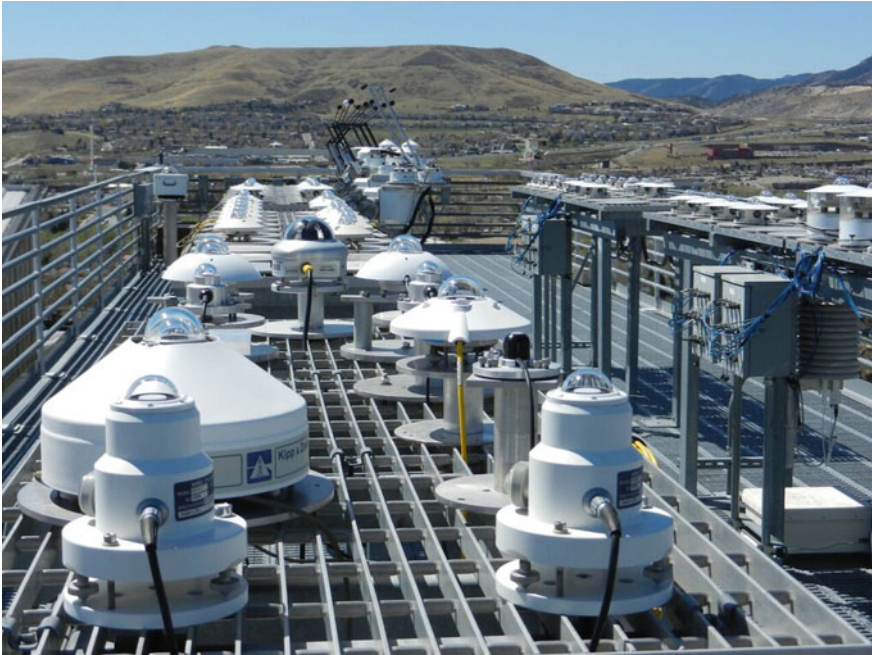
Fig. 7 Solar radiation monitoring platform of the Solar Radiation Research Laboratory (SRRL) at NREL looking to the west. A variety of irradiance instruments are on the left. Toward the west end of the platform, several automatic trackers make DNI and DIF measurements. A second set of shelves on the right support pyranometers undergoing testing or calibration. The platform and tables are gridded to minimize the accumulation of snow. The platform is on the west side above an office building for the SRRL complex. Photograph courtesy of Tom Stoffel
