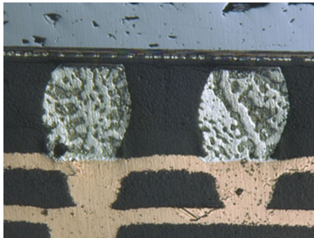
Fig. 27.5 Polished first level solder bumps viewed at 1000× magnification
