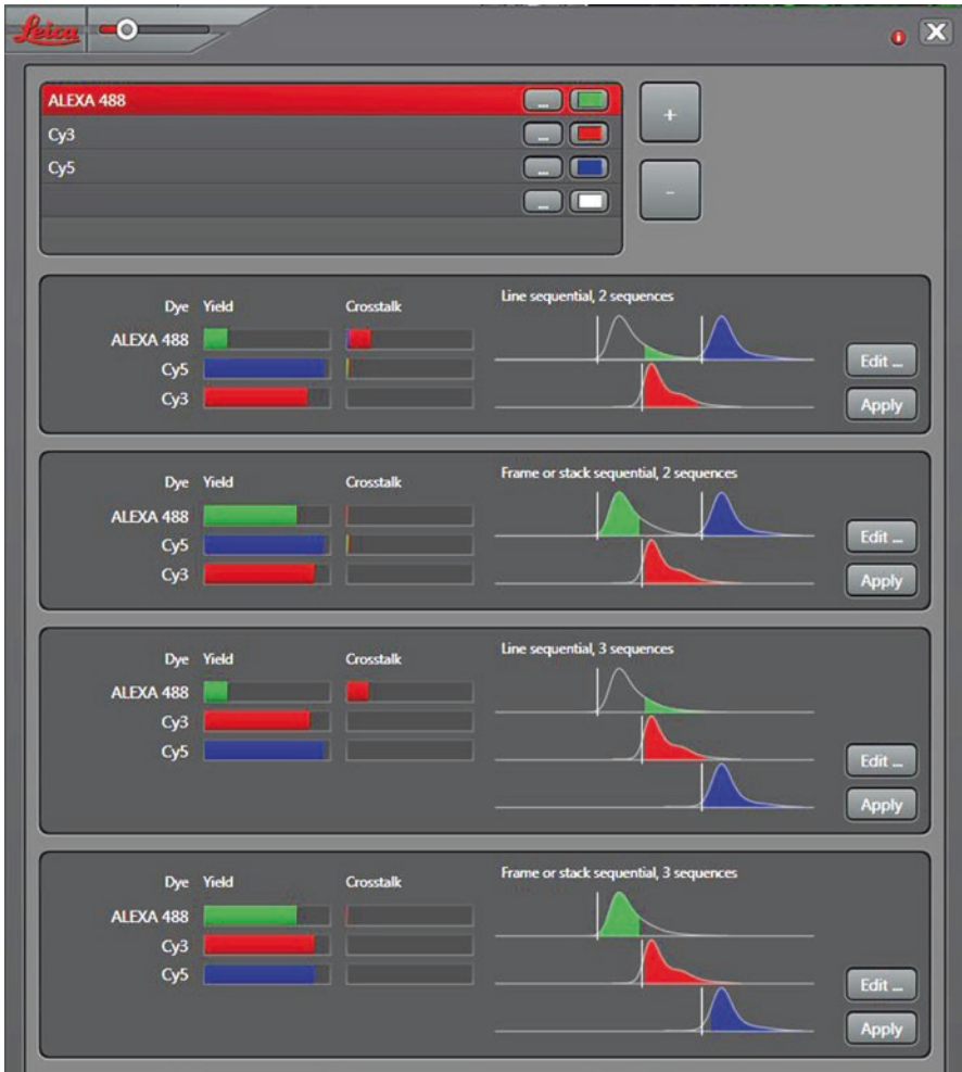
Fig. 9.41 Use of the “Dye Assistant” to establish a sequential imaging protocol for Alexa 488, Cy3, and Cy5
