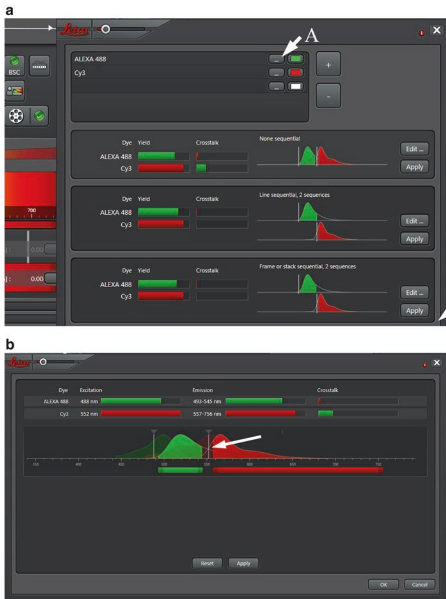
Fig. 9.38 (a) The “Dye Assistant” can be used to add fluorochromes to a protocol by selecting the three dots (arrow A) to open a list of dyes. Each dye can then be assigned a color for an image by selecting the box to the right of the arrow and using a lookup table. When more than one fluorochrome is selected, the “Crosstalk” between the emission spectra will be displayed in the windows under the dye list. The top window shows overlap if “None Sequential” (simultaneous) imaging is chosen and the bottom windows the “Crosstalk” for “Line Sequential” or “Frame or stack sequential.” If “Edit” is selected, a window will open showing the emission spectra superimposed on a wavelength scale. (b) Significant overlap (arrow) exists if “None Sequential” is chosen as the imaging mode. (c) Overlap can be eliminated if “Line Sequential” or “Frame or stack sequential” is chosen
