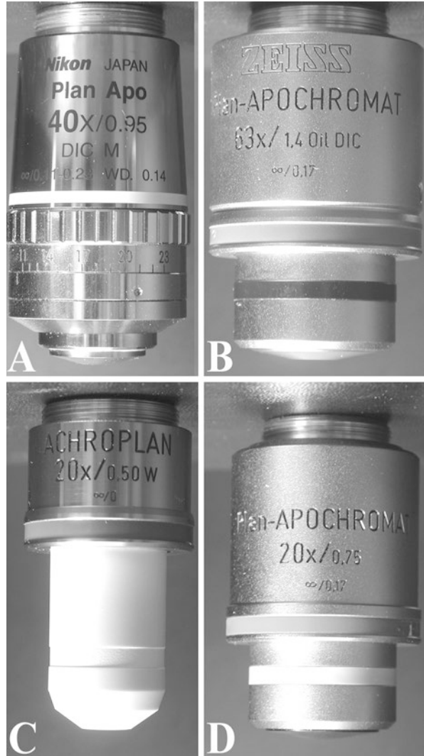
Fig. 3.6 Various types of objective lenses showing inscriptions on the barrel of the objective. (a) 40X Plan Apo with correction collar for adjustment to correct for coverglass thickness and refractive index mismatch; (b) 63X Plan Apo oil immersion; (c) 20X Plan Achromat water immersion; (d) 20X Plan Achromat
