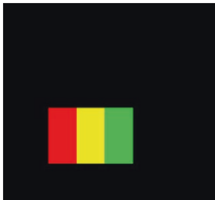
Fig. 11.7 Effects of intensity variability on Pearson's correlation coefficient. Two identical-sized objects (red and green) are shown here with 50% area overlap. These two objects have homogeneous pixel intensity with no variability, thus contributing to a zero value in the denominator for Pearson's correlation coefficient, rendering the calculation impossible. This is an example where co-occurrence of signals does not translate into correlation
