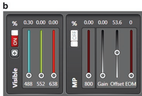
Fig. 9.4 Opening screen of the LAS X software. Overview of the software in the Acquire menu (a). From this window it is possible to access the Configuration, Process, Quantify, Analysis, and Materials windows. (b) The visible lasers are accessed by selecting the “+” button indicated by arrow B
