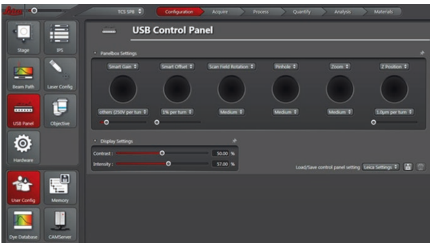
Fig. 9.14 “USB Control Panel” window. Each knob is assigned a parameter by selecting from the top dropdown menu, and the sensitivity of each turn is set with the bottom dropdown menu
