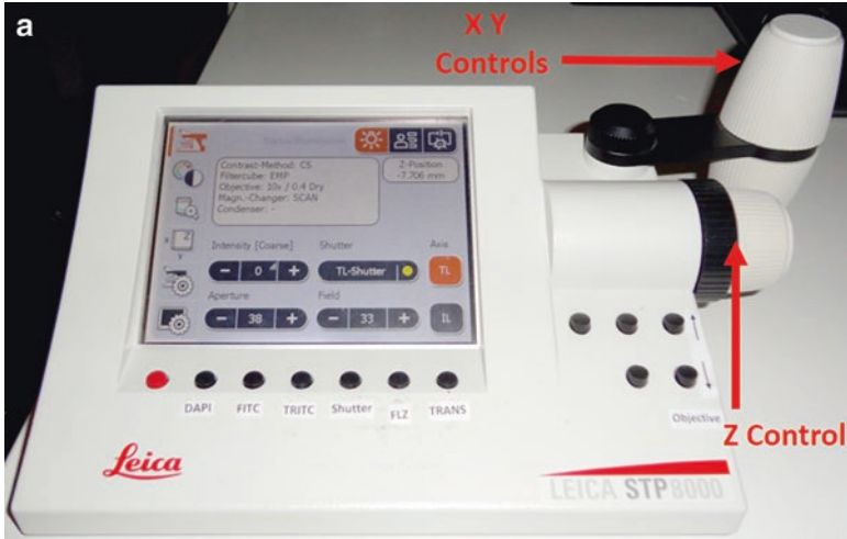
Fig. 9.6 STP8000 Microscope Control Panel. (a) Overview of the control panel indicating XYZ stage and imaging controls. As each icon on the far left of the window is selected, additional microscope functions can be accessed. (b) Selection of “microscope” image on top left allows adjustment of light intensity, Condenser Aperture settings, and field of view and the shutter. (c) The “Color Wheel Icon” allows viewing of the specimen in brightfield (BF), fluorescence (FLUO), or a combination of the two (CS) modes. (d) The “Objective Icon” allows selection of the available objectives on the system by simply touching the objective of choice. (e) The x, y, z icon provides stored parfocality positions for the objective focus (Z) and the X, Y stage position. (f) The “Microscope/Wheel” icon allows setting of various functions for the black buttons on the bottom of the Microscope Control Panel as shown by the DAPI, FITC, etc. labels. These functions can be changed in this window to customize a microscope. (g) The “Monitor/Wheel” icon allows calibration of the Control Panel
