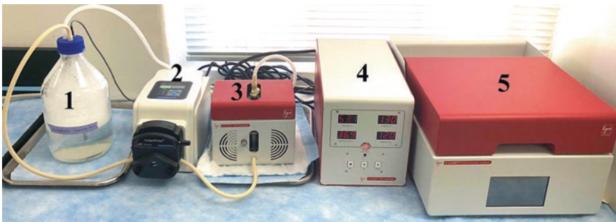
Fig. 4.6 Components of the Logos Biosystems X-CLARITY™ tissue clearing system. (1) Chemical reservoir for clearing fluid exchange, (2) pump to transfer clearing fluid from the chemical reservoir to the electrophoretic clearing (ETC) chamber, (3) ETC clearing chamber, (4) control unit for setting time and temperature of the ETC unit during clearing, (5) hydrogel embedding and polymerization unit
