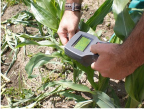
Fig. 17.3 Determination of fluorescence parameters: QUANTUM efficiency of photosystem II (ΦPSII) by using a portable OS-30p Chlorophyll Fluorometer (Opti-Sciences, Tyngsboro, Massachusetts, USA)
