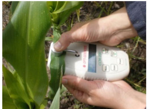
Fig. 17.2 Determination of chlorophyll content (SPAD units) using a hand-held CCM-200 Chlorophyll Content Meter (OptiSciences, Tyngsboro, Massachusetts, USA)
