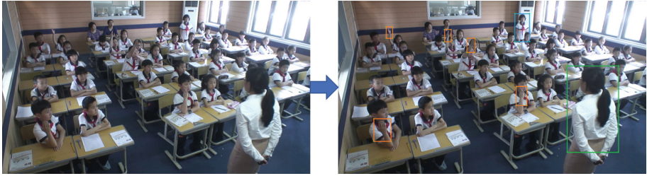
Fig. 1. The learning-and-teaching related behaviors detection is converted into a frame-based standing (blue box), hand-raising (orange boxes) and teacher (green box) multi-object detection. (Color figure online)
