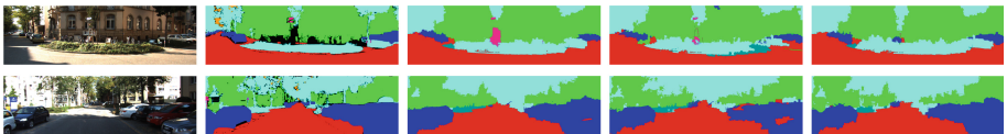
Fig. 4. Segmentation visualization of KITTI examples. The first column shows two inputs. The second column shows the groundtruth. The rest columns, from left to right, are results by Adj-CRF, MST-CRF and LG-CRF respectively.
