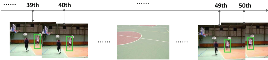
Fig. 1. This is a detection result when a shot change occurs. No action is detected due to the shot change after the 40th frames until the 49th frame, and the number of undetectable frames exceed the threshold, so the formed action tube is interrupted. However, the action is still in progress. From the 49th frame, a new tube is generated again because the camera switched back and detected the previously unfinished action. Those two sub-action tubes belong to a same action event.
