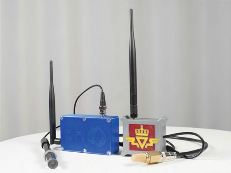
Fig. 2 Two IoT weather and environment sensors developed in our laboratory in cooperation with Telenor and their Start IoT initiative: a pH sensor to the left and a humidity sensor to the right (picture from Telenor)
