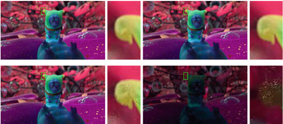
Fig. 5. Rendered scene of the worm with filtering; from left to right, up to bottom - 512 samples/pixel, 256 samples/pixel, 64 samples/pixel, 1 sample/pixel
