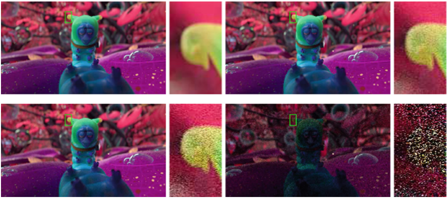
Fig. 3. Rendered scene of the worm without filtering; from left to right, up to bottom - 8196 samples/pixel, 256 samples/pixel, 64 samples/pixel, 1 sample/pixel
