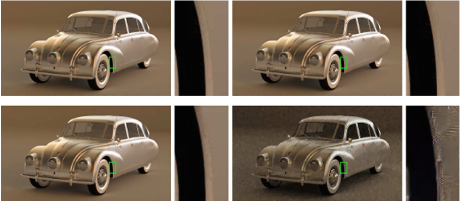
Fig. 4. Rendered scene of Tatra car with filtering; from left to right, up to bottom - 512 samples/pixel, 256 samples/pixel, 64 samples/pixel, 1 sample/pixel
