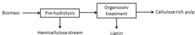
Fig. 2 Schematic of a combinative organosolv pretreatment
