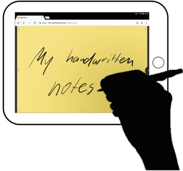
Fig. 3 Schema of the MED-Pad web application on a tablet device. Hand drawn scribbles on a full-screen surface are converted into their corresponding textual representation at the user's command
