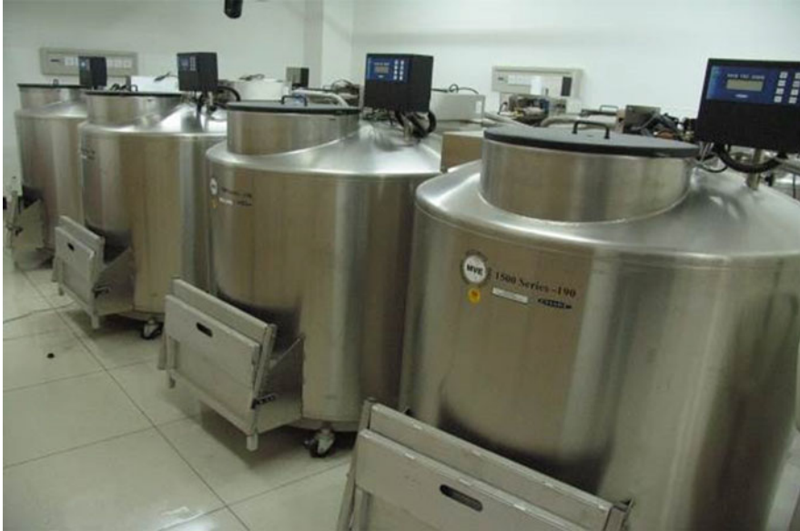
Fig. 3.3 Liquid nitrogen tanks
