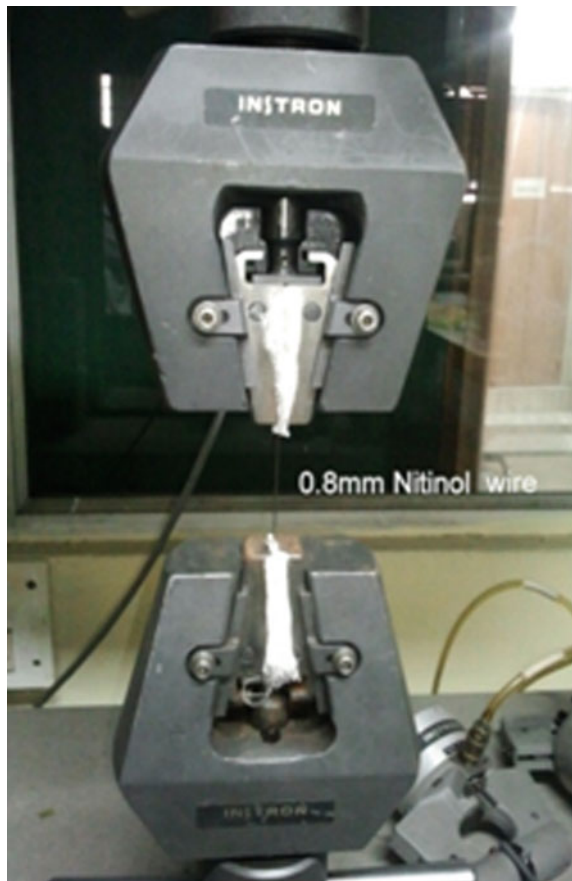
Fig. 8.2 Arrangement for tensile testing (arrow shows the padding used for holding Nitinol wire)
