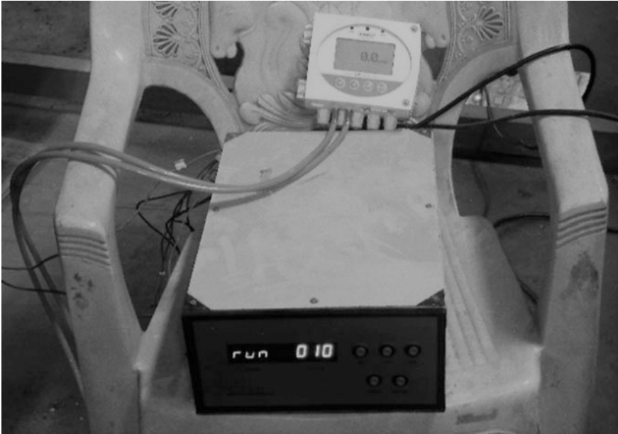
Fig. 31.4 Robotic arm controller with digital manometer on top of it
