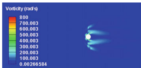
Fig. 32.22 Vorticity at \varepsilon = 1 and w = 0.75 for reacting flow
